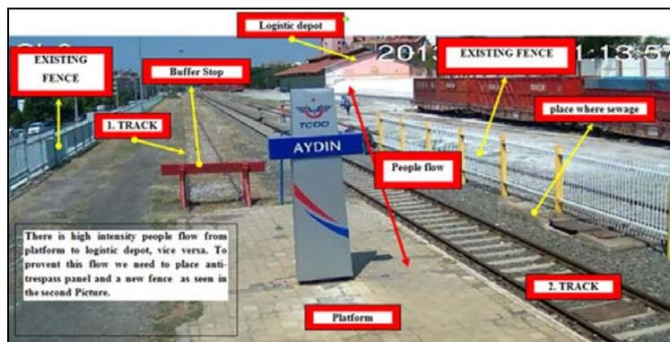
**Figure 5.5-5: Measure 7: Installation of anti-trespass panels in the first point.**
