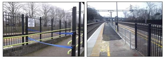
Figure 5.6-3: Example of some temporary fencing that is obstructing access to the fast line platform (left). Examples of two types of fencing that were provided for reasons other than fatality prevention (right).
